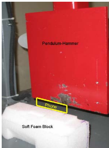
Figures 1a (left) and 1b (right). Test configuration and strain gage on PWB of cell phone.
