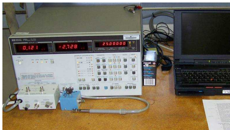
Figure 9 – Setup of the Virginia Tech SHM instrumentation.
