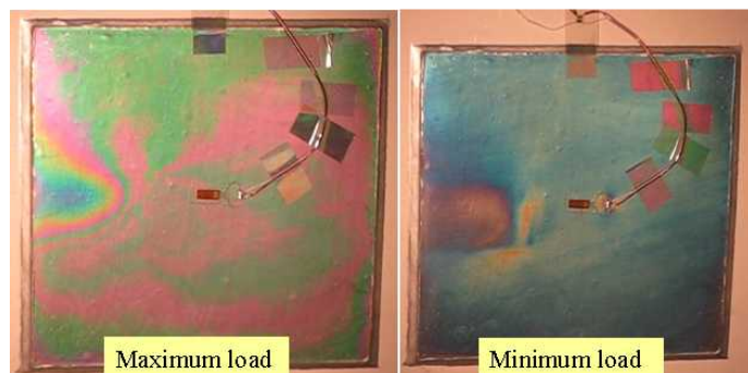
Figure 22 - Two snap-shots (at maximum and minimum fatigue load) of the photoelastic panel on the low pressure, compression, downward facing, blade surface over the spar cap termination point at 4.5 meters. Note the high strain gradients around the termination point of the spar cap.
