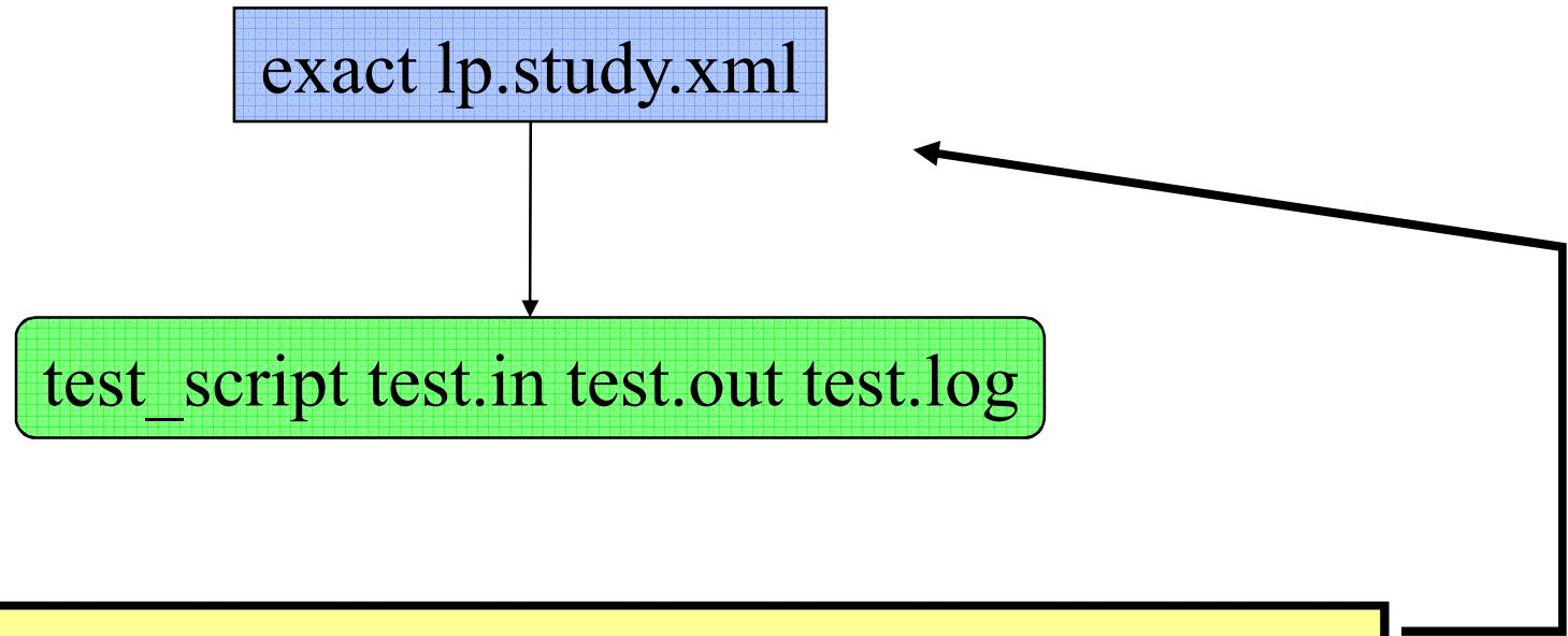
The EXACT script launches a user-defined script to execute each experimental treatment. Measurements are extracted from the \*.log file to generate a \*.out file.
