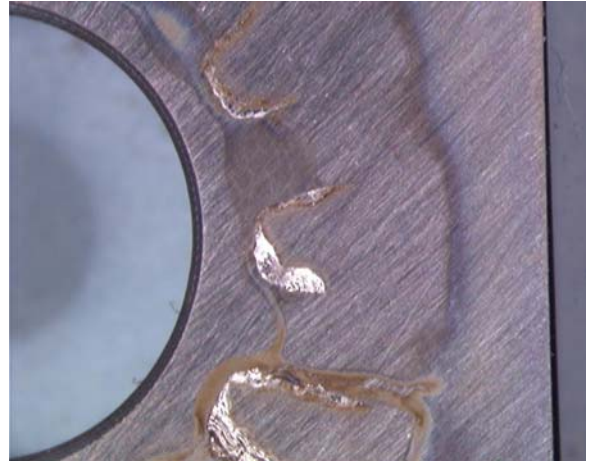
Figure 8. Specimen HH001 after the CPP test
