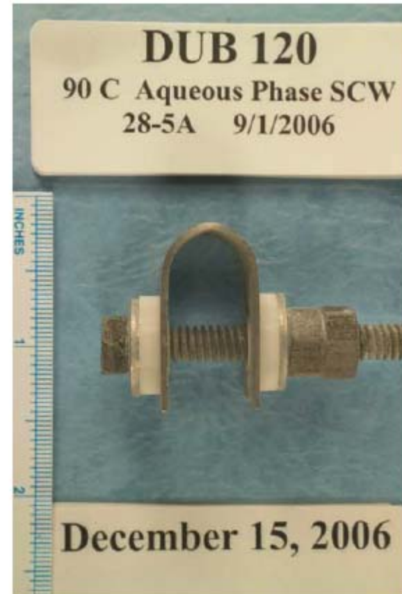
Figure 6. Alloy 22 U-Bend specimen tested for 9.3 years in SCW at 90°C. No cracking
