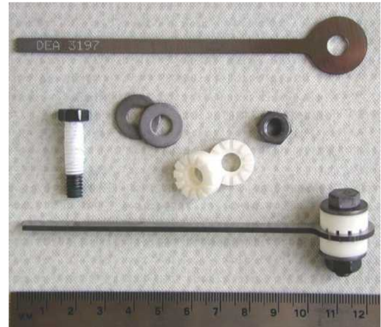
Example of a specimen configuration used for electrochemical testing. Other configurations were also used.
