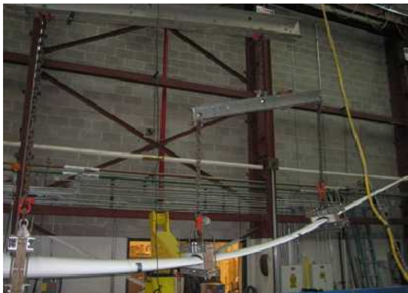
Figure 3. Static Test on the BSDS Wind Turbine Blade
