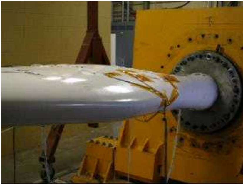
CX-100 Dimple (left) and Tip Movement (right) just before Failure
