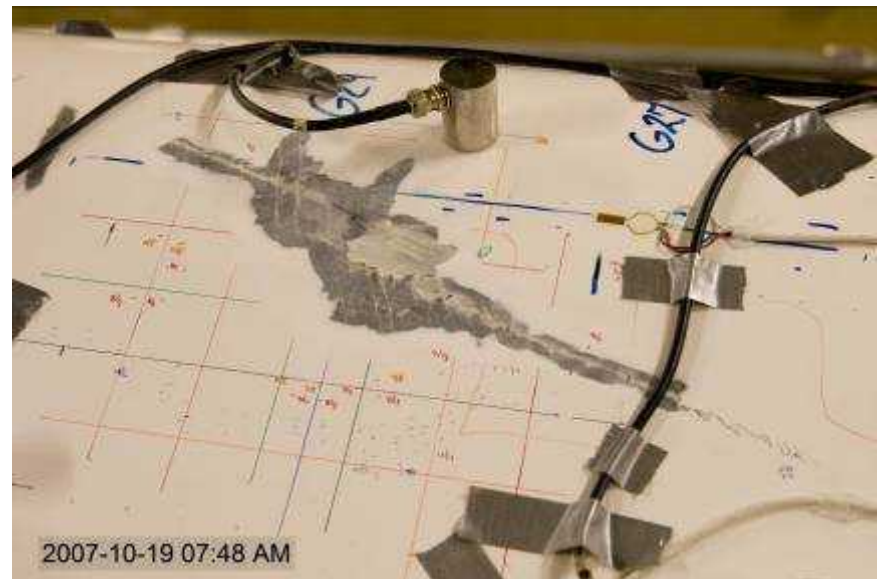
TX-100 Crack Growth Beginning (left) and Progression (right)
