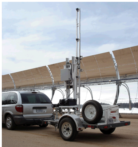
Figure 5. The TOP alignment system can potentially reduce facet alignment errors to 0.5 mrad.
