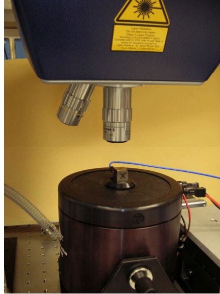
Figure 3: An accelerometer was mounted on a shaker. The LDV laser beam sensed the velocity through the microscope optics. In a different test setup (not shown), the LDV laser beam sensed the velocity without a microscope.
