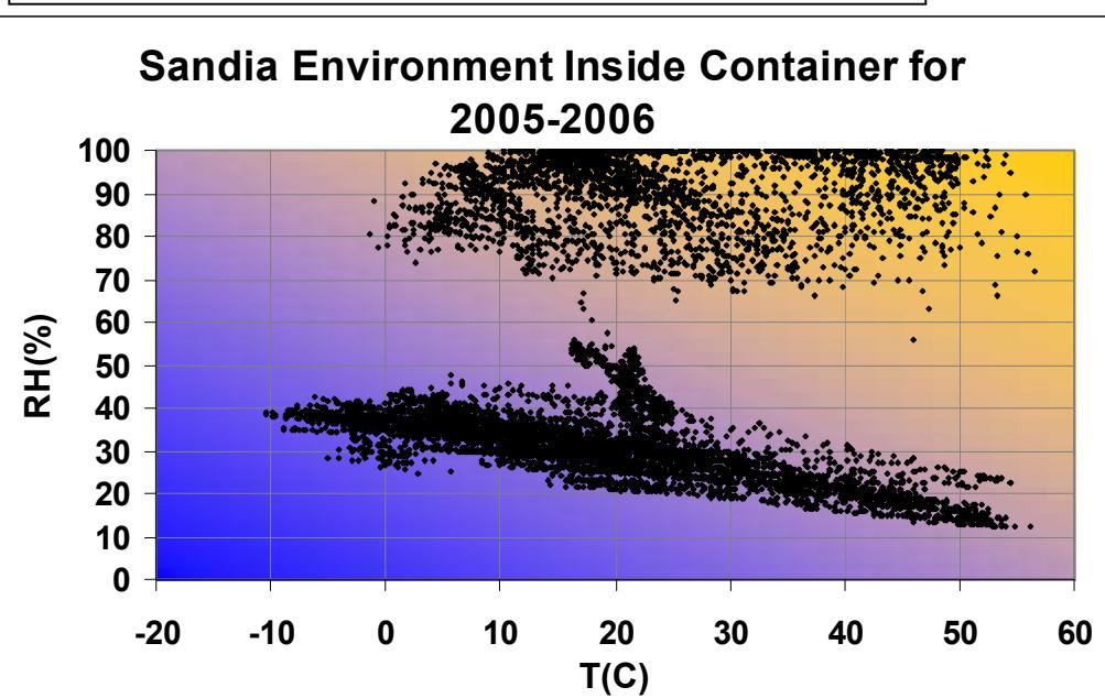
$$AF(s, s_0 | Q_a, n) = \exp \left[ \frac{Q_a}{k_B} \left( \frac{1}{T} - \frac{1}{T_0} \right) \right] \left( \frac{RH_0}{RH} \right)^n$$
