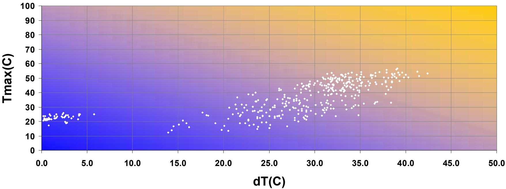
Severe environments leading to short predicted lifetimes correspond to data points in upper right corner. Benign environments/long lifetimes correspond to lower left corner.
