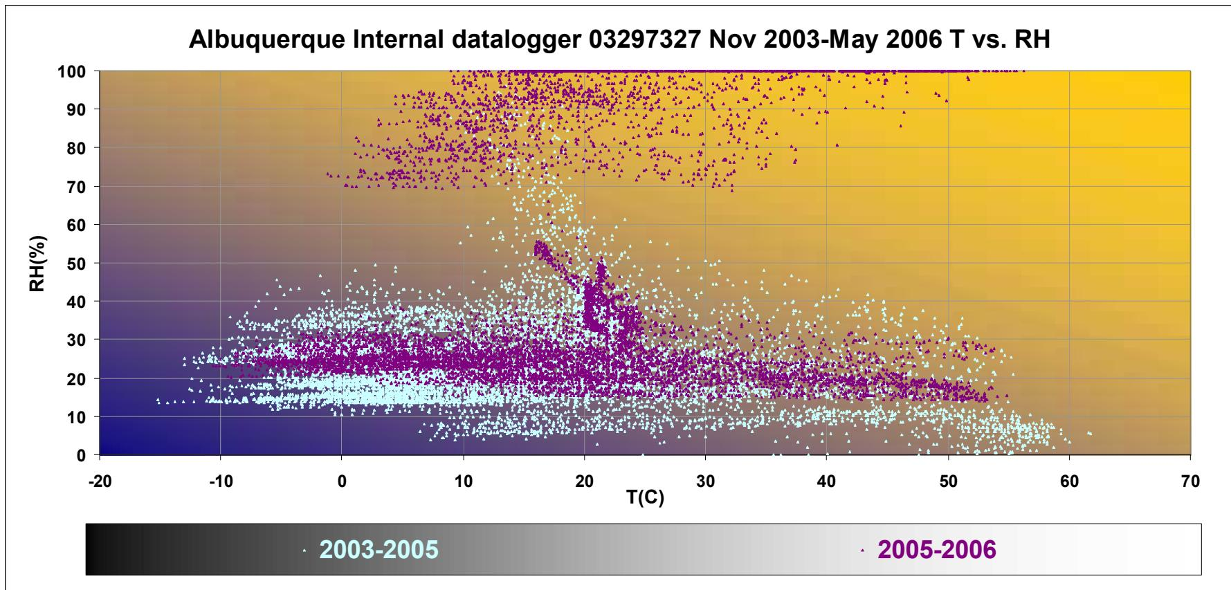
Severe environments leading to short predicted lifetimes correspond to data points in upper right corner. Benign environments/long lifetimes correspond to lower left corner.
