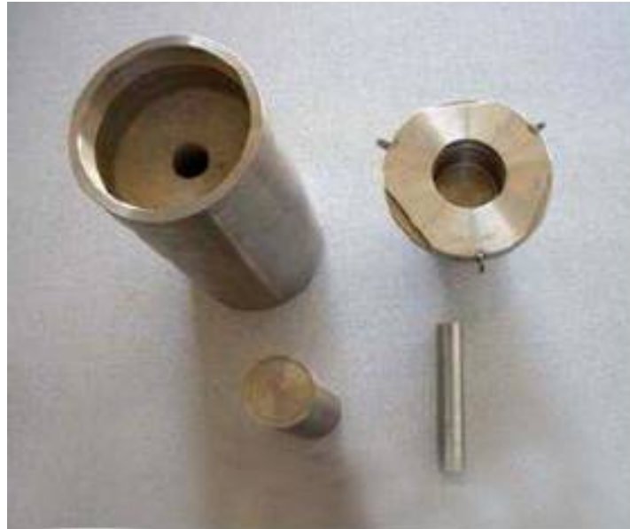
Photograph of the BOSS Outer Disposal Container (11 cm in diameter) with the Two Sizes of Inner Capsules on the bottom of the Photograph (from IAEA, draft, 2006)
