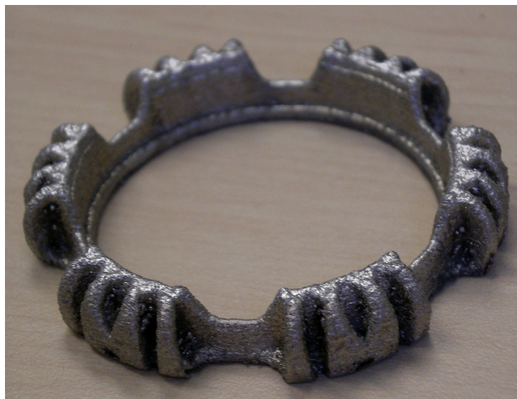
Figure 17. Prototype component manufactured from STL file.
