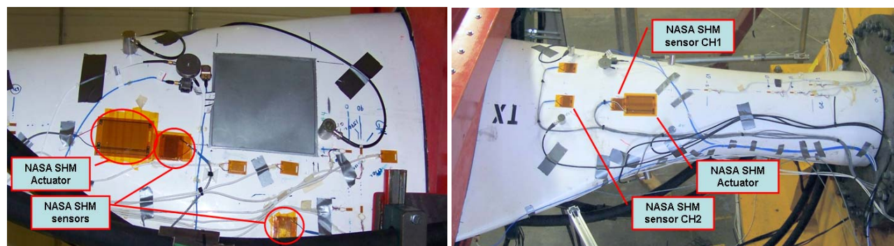
Figure 6 – Photos of the NASA SHM sensor arrays. The left photo shows the low-pressure (downward facing) side of the blade. The right photo shows the high-pressure (upward facing) side of the blade. The larger MFC patches were used as actuators, the smaller MFC patches were used as sensors.
