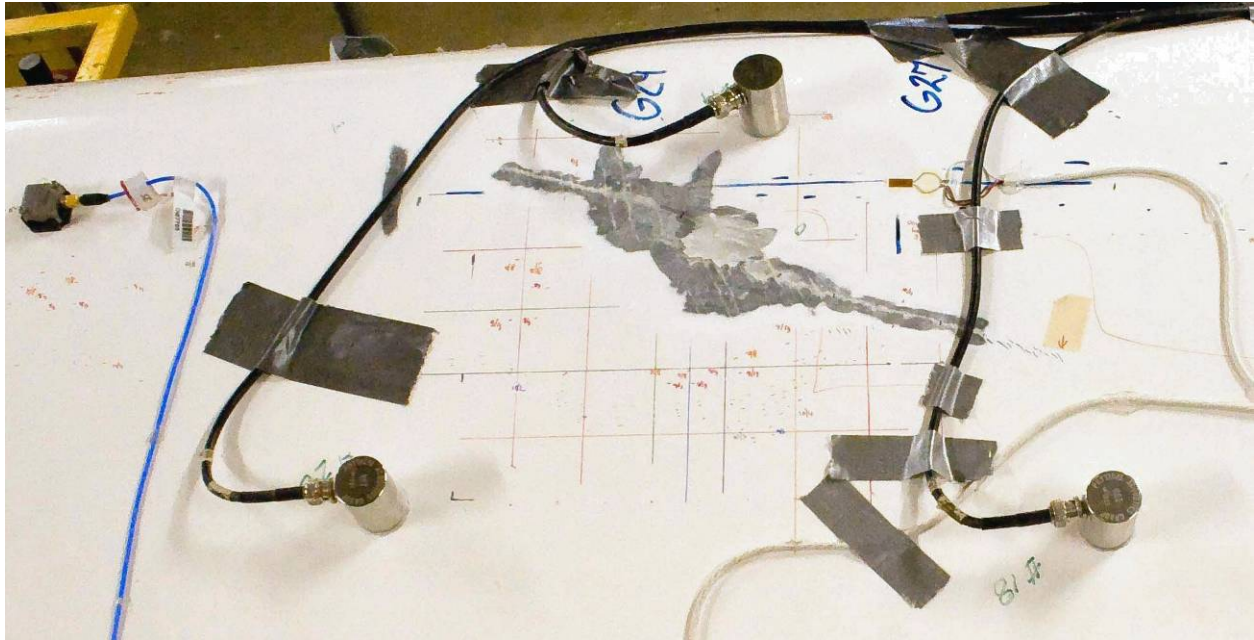
Figure 11 – Photo showing the blade surface around the area of failure. Some of the gel-coat has been manually removed to better evaluate the underlying damage.
