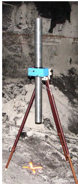
Figure 2 Sandia dipole antenna in vertical polarization inside underground cavity.
