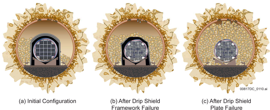
Figure 3. Artist's interpretation of the changes in the underground structure of the repository modeled in the Total System Performance Assessment: drip-shield failure and rock falls in response to accumulating damage from earthquakes
