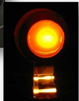
Four pocket rotary turret 10kV electron beam gun, and molten material during deposition
