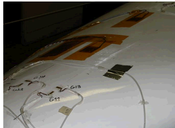
Figure 25: CX-100 low-pressure skin damage area.
