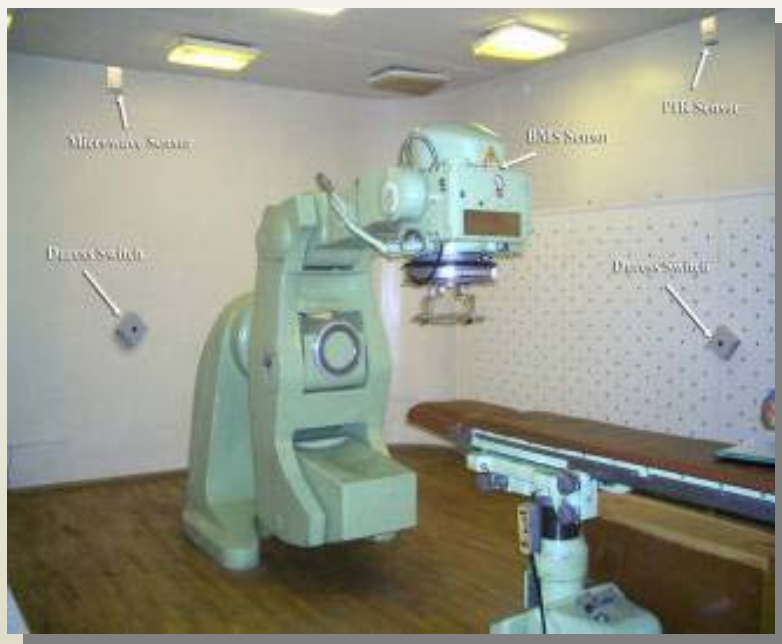
Oncology clinic security enhancements include installation of sensors to detect entry into room that holds source and sensor on the teletherapy unit itself.
