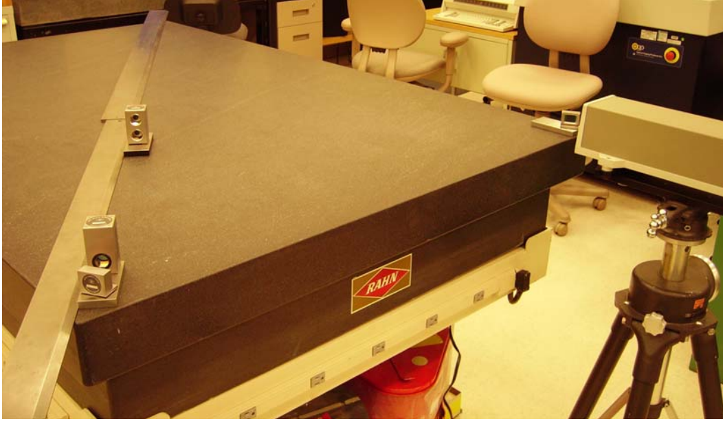
Figure 11: Set-up for laser interferometer calibration
