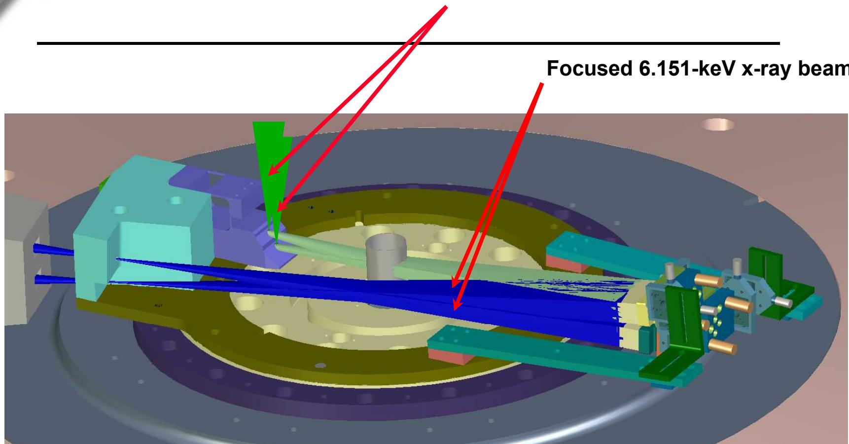
Each of the two image-plane detectors (*Image Plate*) capture one time-integrated image
