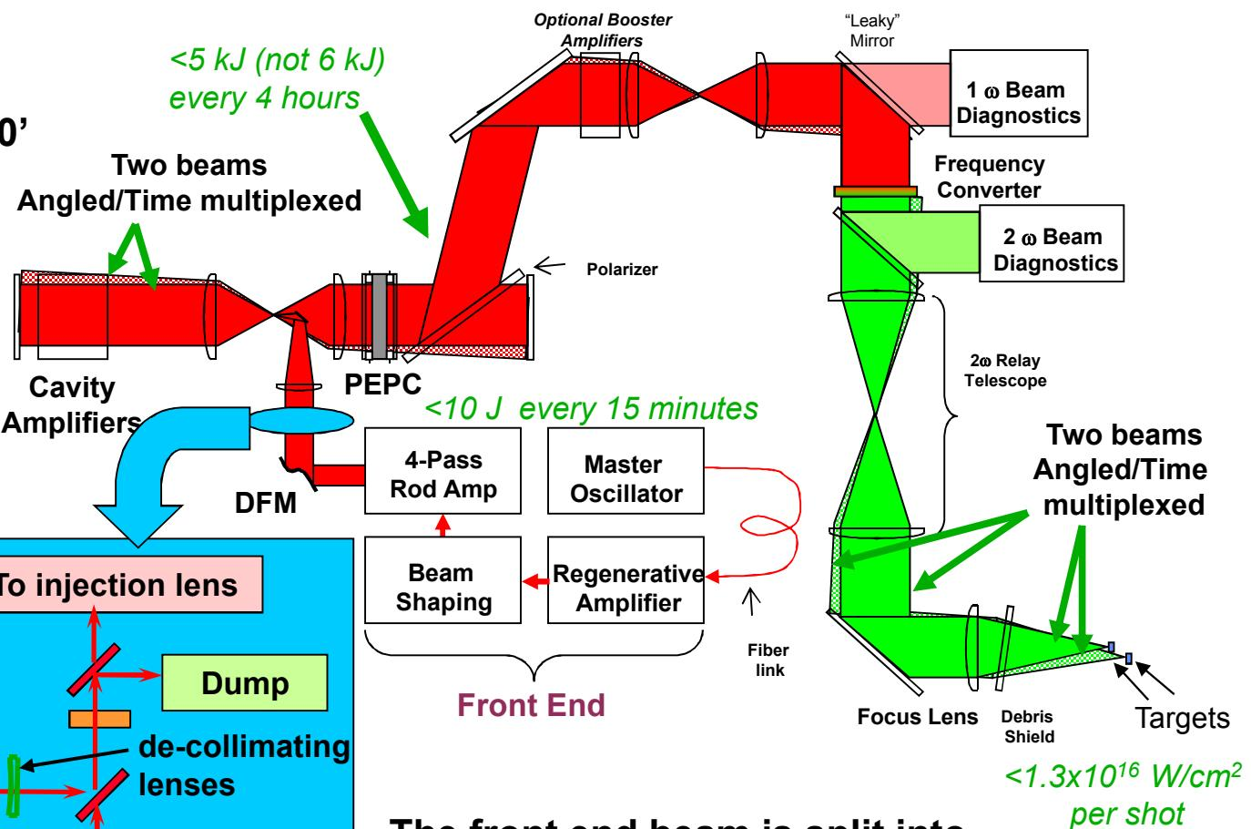
The front end beam is split into Two, with variable energy ratio
