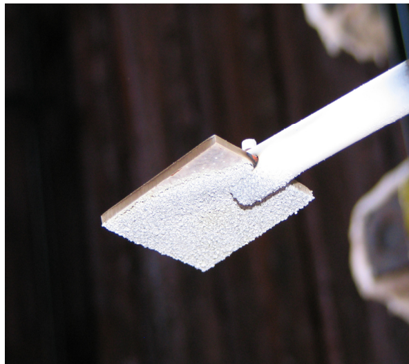
Figure 2: Copper coupon after sample collection
