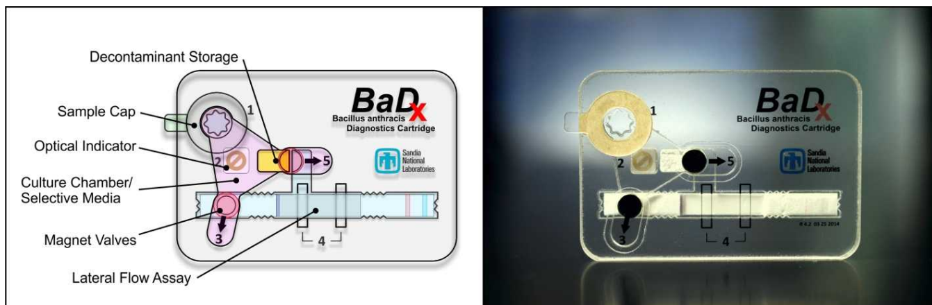
Figure 1. Left ; Schematic of cartridge showing major components. Right ; Photo of the fabricated cartridge with dimensions of 0.25 in. x 1.875 in. x 2.75 in.
