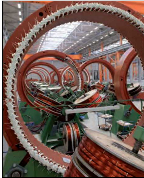
Enercon's wire-wound-rotor direct-drive generator has no gear box and requires no rare earth magnets but offshore deployment is hindered by the limited service lifetime of rotary electrical contacts.
