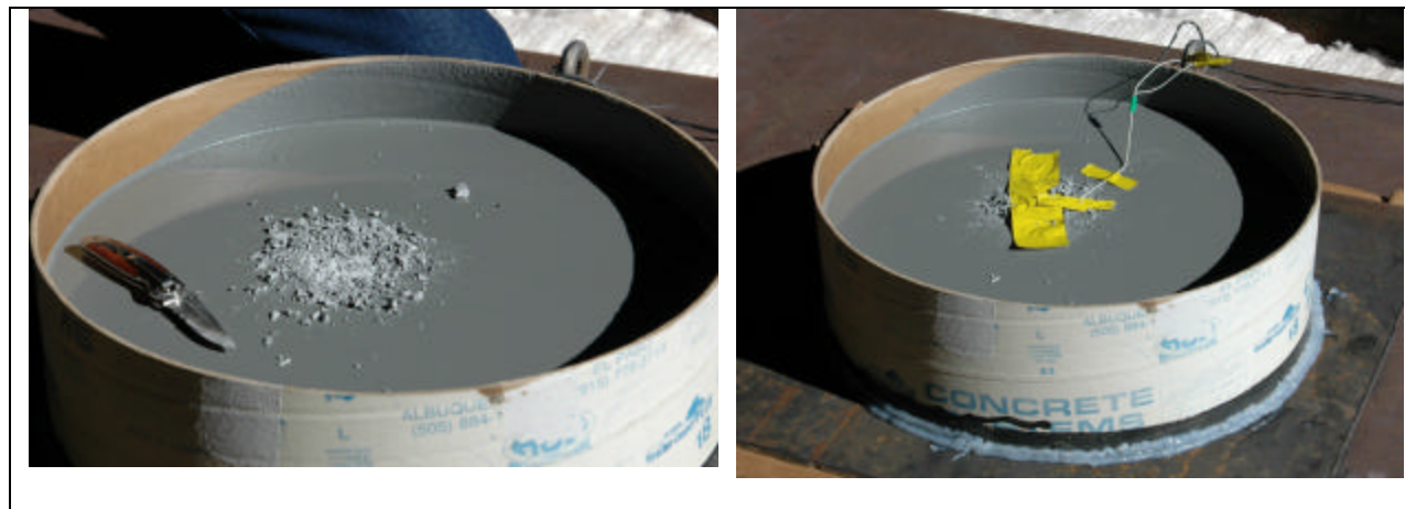
Figure 4. A 20" dia propellant sample with cardboard side inhibitor. The ignition charge is propellant crumbles and an electric match.
