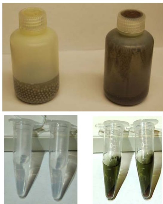
Fig. 6. Bottles from the tumble test containing stainless steel balls (left) and copper balls (right), after tumbling for 12 hours. Samples of the fluid were centrifuged in the vials below to extract solid particles for analysis.
