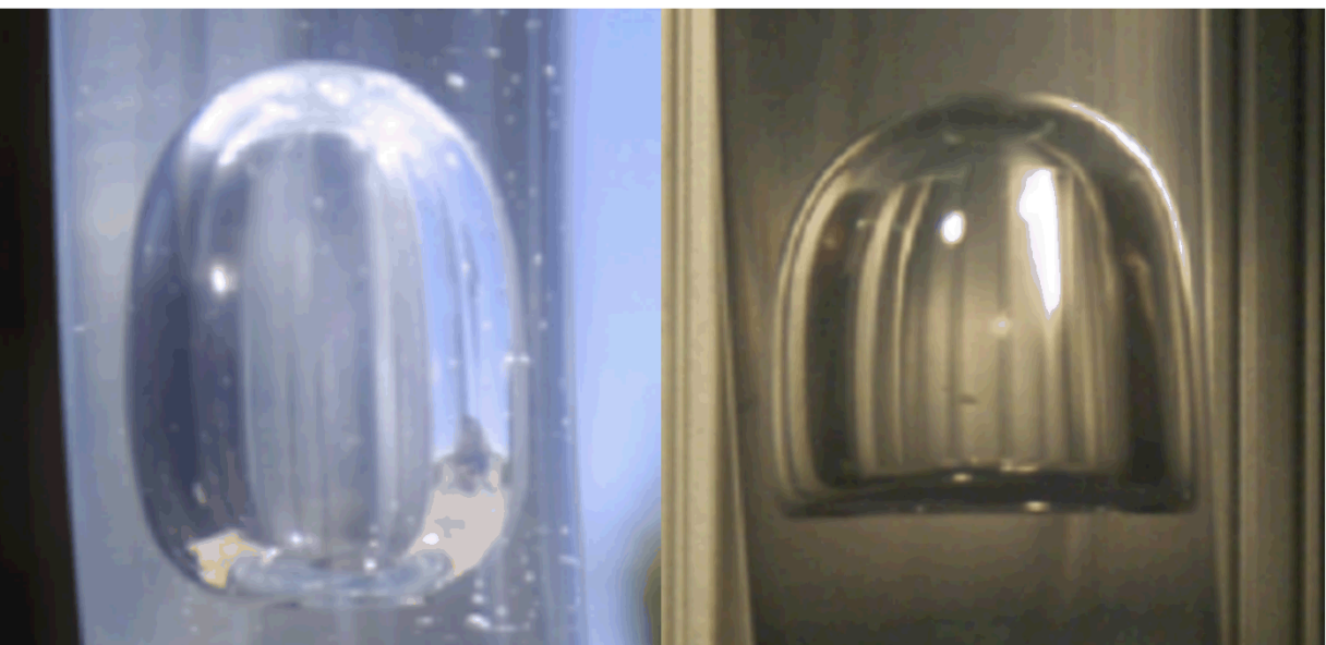
Figure 8: Bubble shape in glycerine (left) and mineral oil (right)
