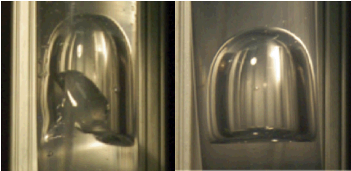
Figure 7: The effect of varying pulse duration and air pressure: on the left is a high-pressure short pulse, and on the right is a low-pressure long pulse
