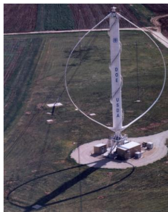
Figure 8. Sandia 34-meter VAWT test bed
