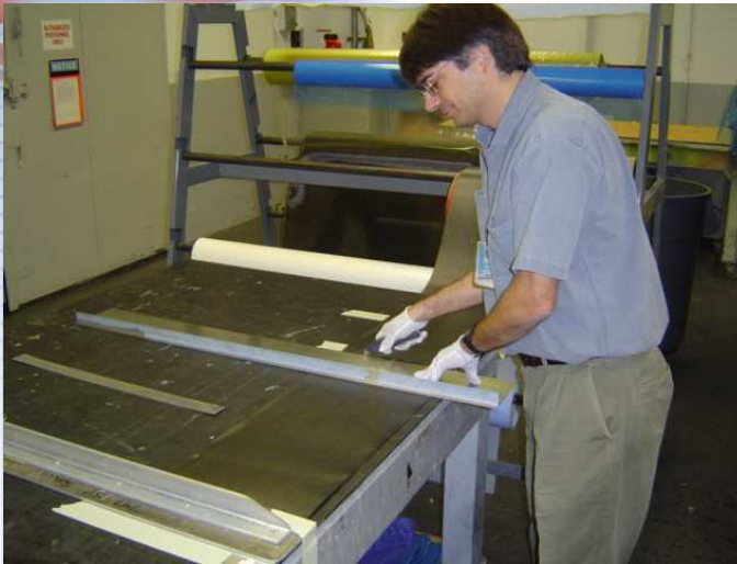
Flaw templates - ensure proper location of flaws
