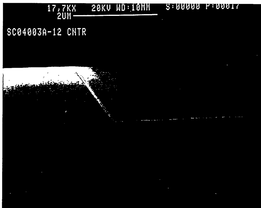
Figure 4. A cross-sectional view of a KOH-etched trench refilled with oxide and planarized using chemical-mechanical polishing. This planar structure is ready for standard CMOS processing.
