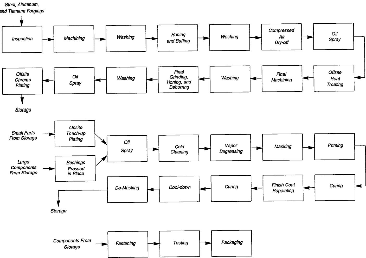
**Figure 1.** Abbreviated process flow diagram for manufacture of aircraft landing gear.
