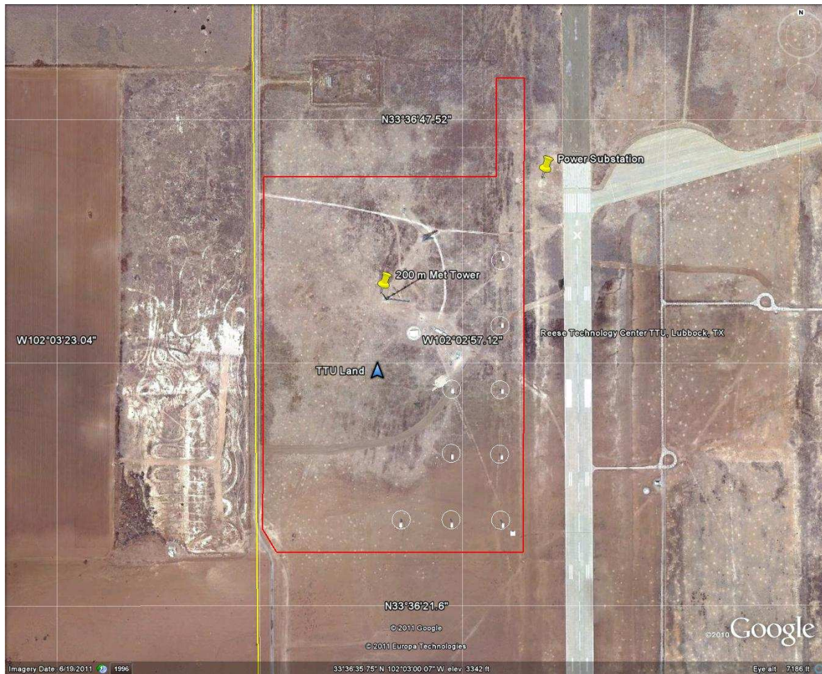
Figure 8. Map of the northwestern portion of Reese Technology Center. The yellow line is the technology center's western border. The red boundary encloses land leased by Texas Tech. The white circles are proposed turbine locations.
