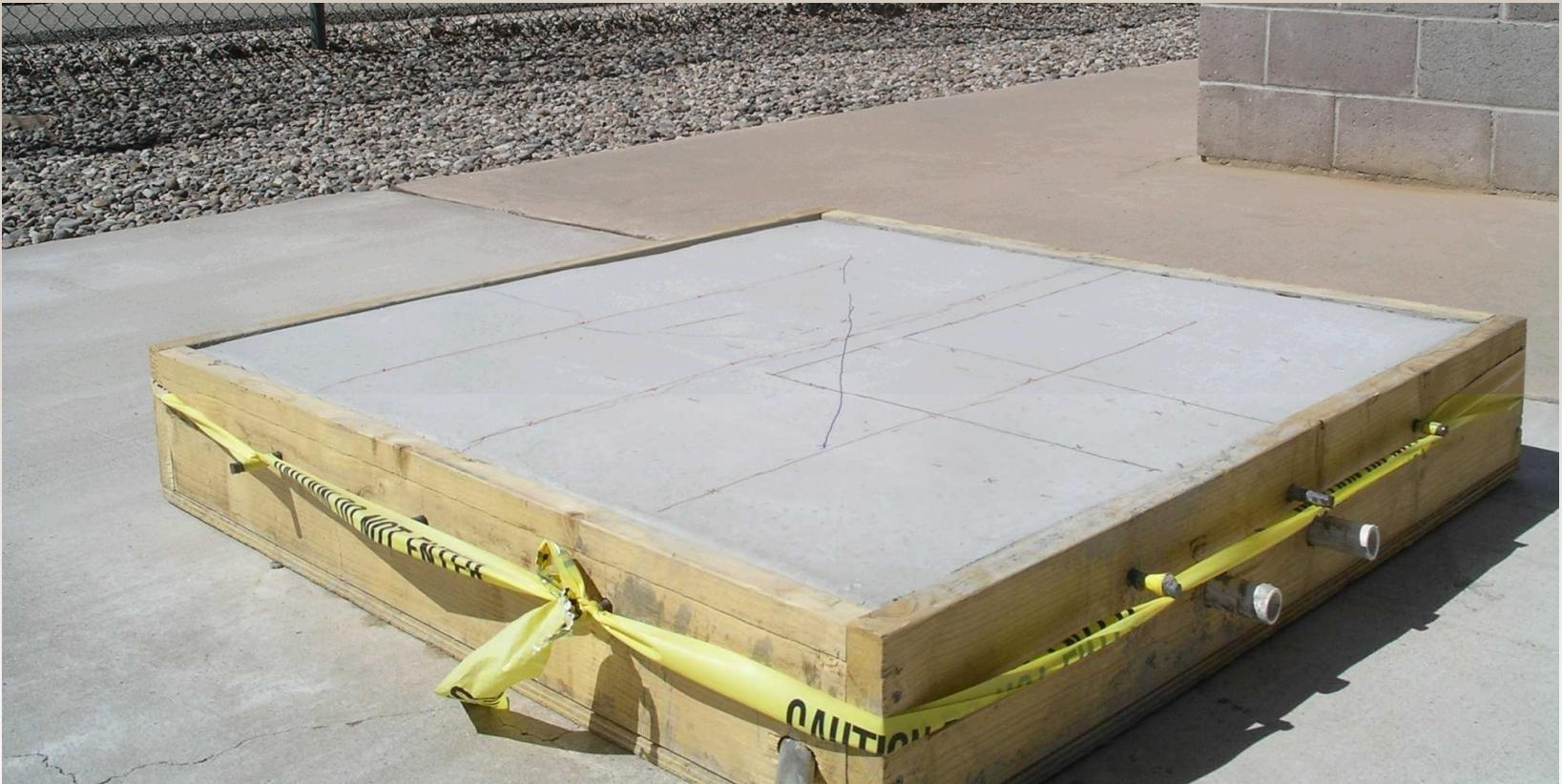
Test block built for testing and calibrating equipment.
