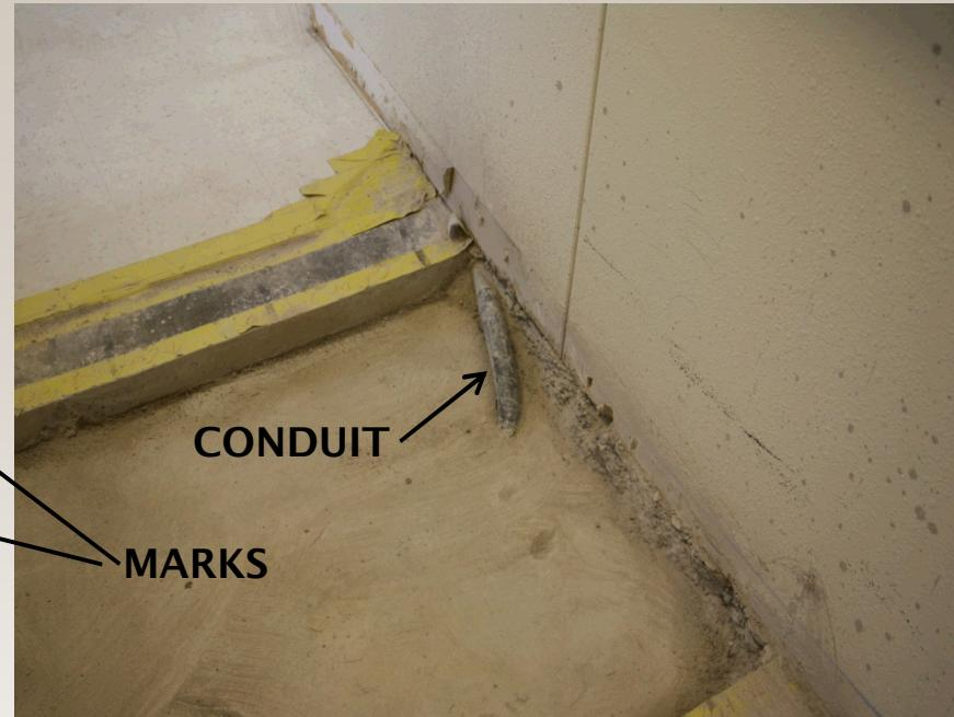
The conduit on the right was identified as an anomaly during the scan and marked in green, but the correct direction the object was traveling could not be identified. Experience should improve the ability to interpret these types of objects, and the palm antenna will help with these types of applications.
