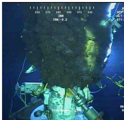
Flow images from the top of the BOP after removal of the kinked riser section (top) and flowing out from Top Hat skirt (bottom)
