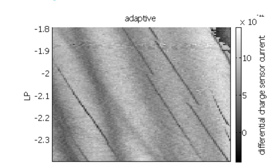
The variation in the quantum point contact sensitivity can mask important features. In this and other devices we can use the dc current through the point contact with software feedback on RQPC to increase the range of sensitivity. While this simple approach assumes the sensor is independent of the dot (clearly not true), more advanced control can be implemented that will maintain high sensitivity.
