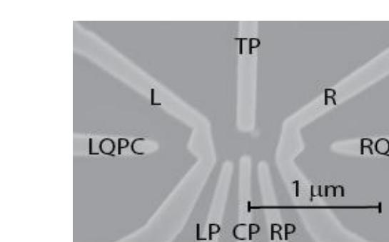
The gate pattern here has 270 nm tunnel and point contact openings. This allows low threshold voltages on the top gate and better control of the dot occupation.
