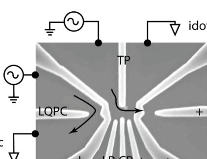
For direct charge sensing, two ac bias voltages with two different frequencies are applied to the dot and charge sense channel. The current is measured resulting in a conductance measurement in each channel.
