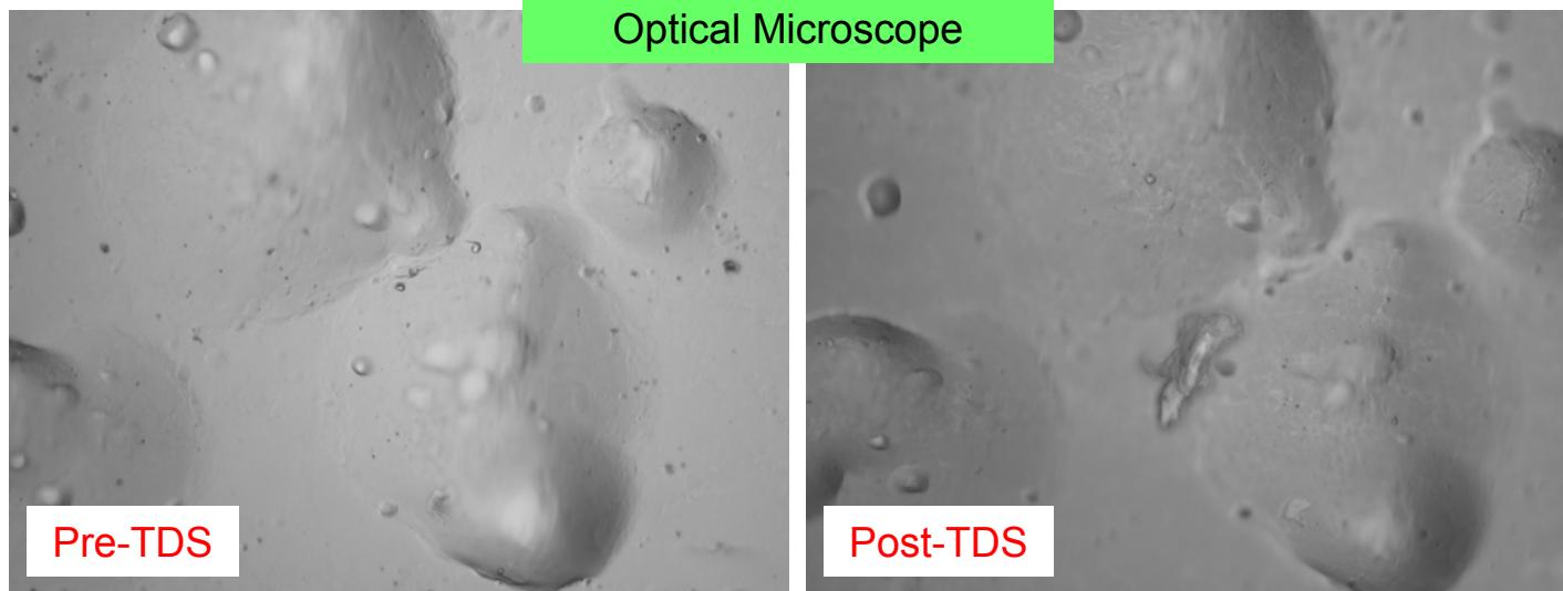
The blisters shown to the left were imaged before and after thermal desorption. There is no conclusive evidence that the blister caps have collapsed, or any other substantial differences emerging due to the desorption process.
