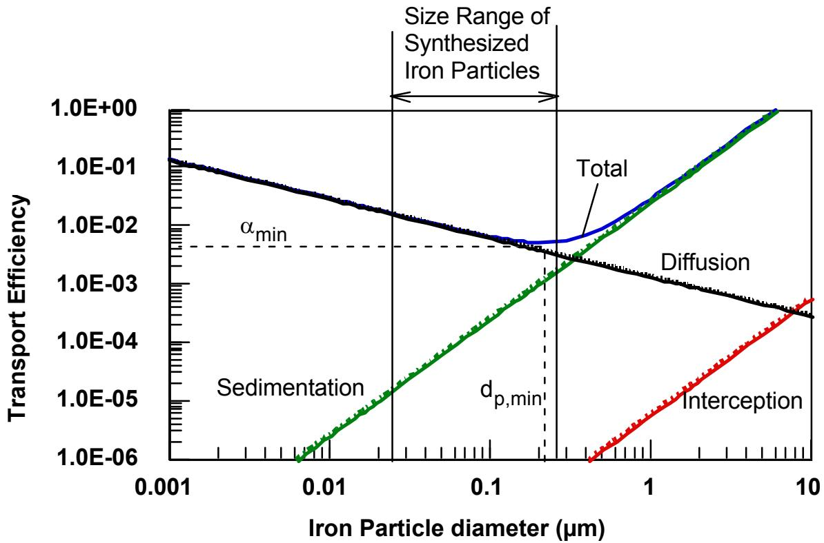
$$\eta = \eta_D + \eta_I + \eta_G = 0.9 \left( \frac{kT}{\mu d_p d_c v} \right)^{\frac{2}{3}} + 1.5 \left( \frac{d_p}{d_c} \right)^2 + \frac{(\rho_p - \rho) g d_p^2}{18 \mu v}$$
