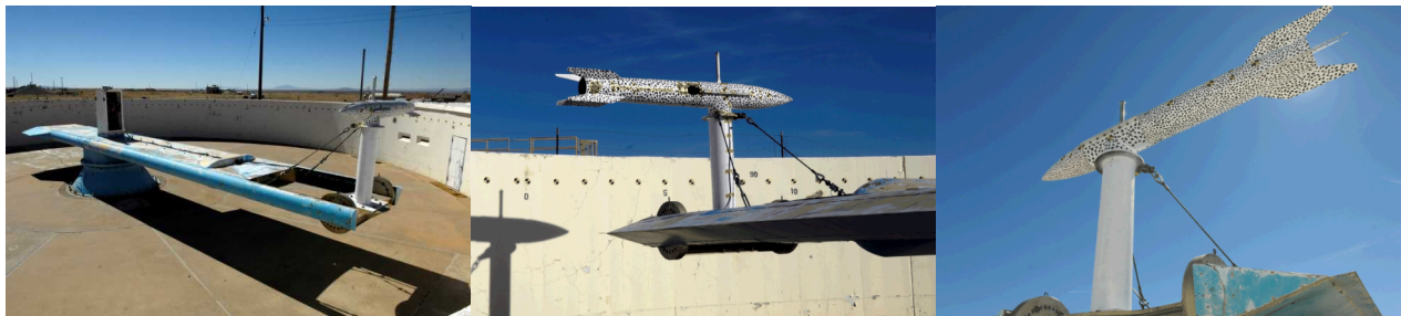
Fig. 2. Speckled test-unit affixed to 10.7 meter arm on the outdoor centrifuge at Sandia National Laboratories
