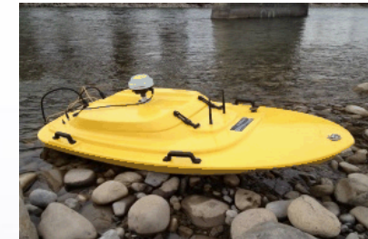
Remotely controlled survey boat with GPS
