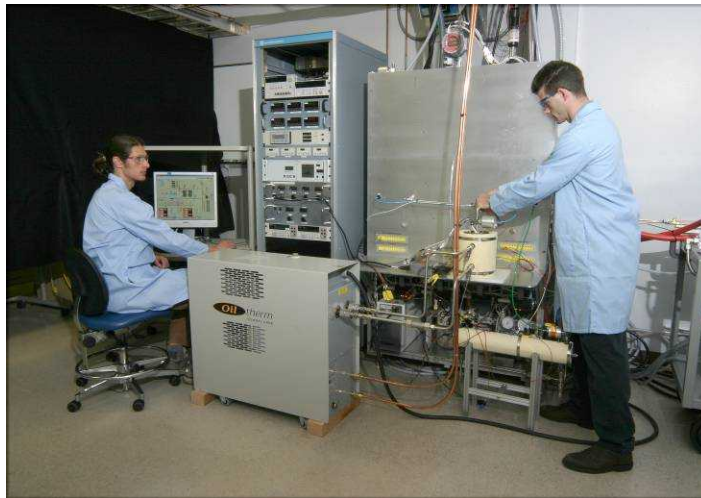
Engineers experimentally validate thermal and chemical kinetic performance of our solid-state hydrogen storage prototype designs.
