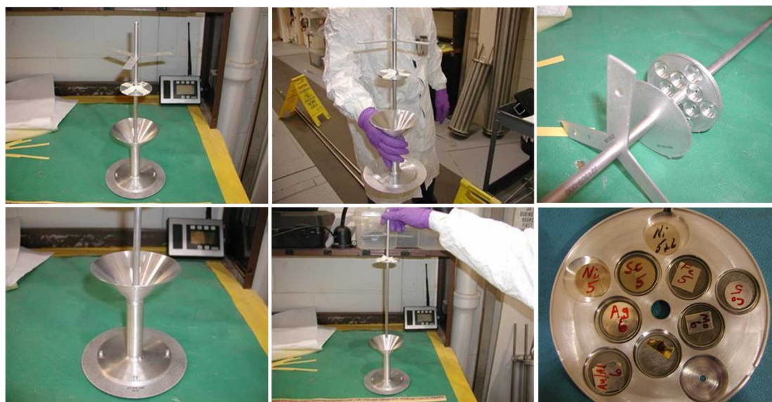
Figure 4. Dosimetry stand used to perform activation foil irradiations at the peak neutron flux
