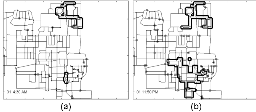
Figure 6. Scan test results for 100 sensing-nodes and 2 contaminant sources. (a) Results when both sources are first detected. (b) Results after 24 hours.
