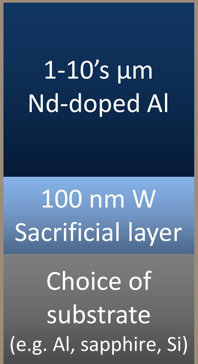
A sacrificial W “valve” layer oxidizes partially through during anodization. The  $\text{WO}_3$  is selectively removed to leave a conductive W layer at the pore bottoms. This facilitates catalyst electrodeposition, even on insulating substrates.
