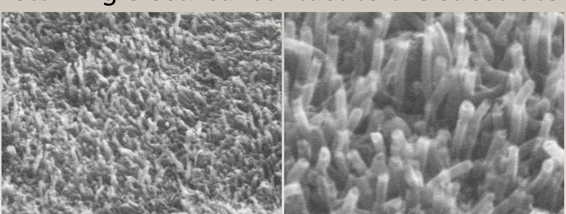
Raman confirms growth of uniform MWNTs. Individual CNTs can be harvested for device fabrication or characterization.
