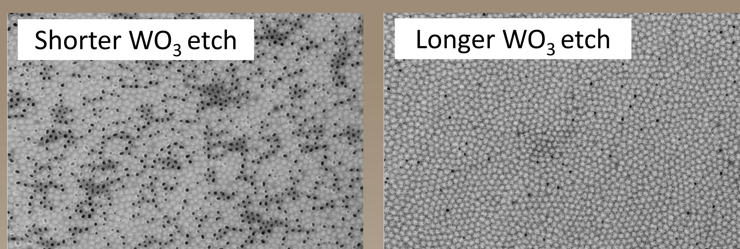
Ion milled pores expose Co catalyst. Empty pores appear dark.
