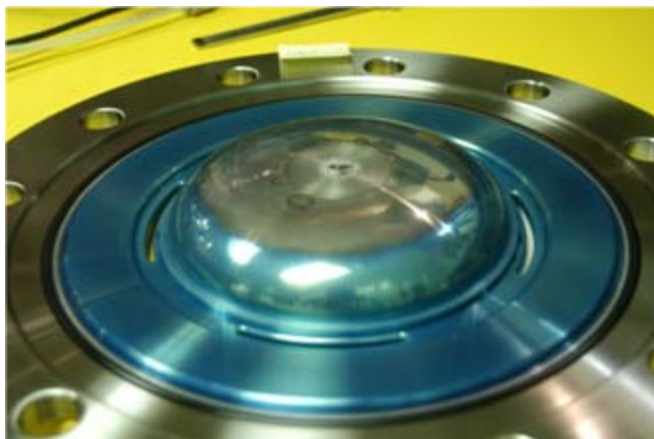
Molybdenum trigger electrodes: byproducts coated insulators and led to flashing (43 shots)
