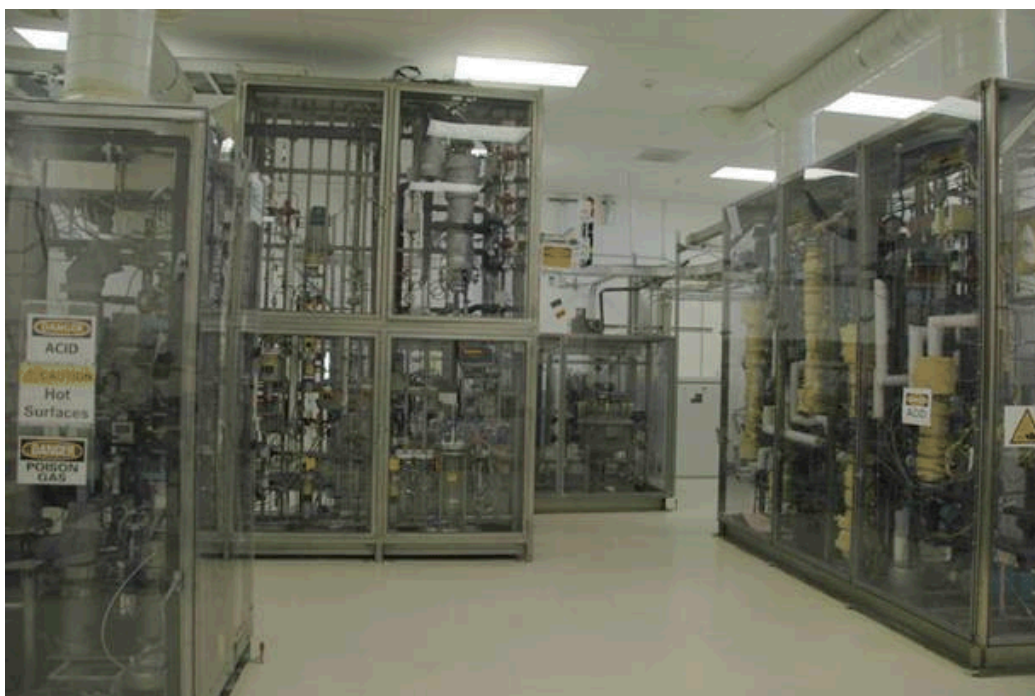
Fig. 4. S-I process showing three chemical process skids and chemical storage skid. From the left, the acid decomposition skid, the Bunsen process skid, the chemical storage skid (only partially visible in the back) and the hydrogen iodine decomposition skid
