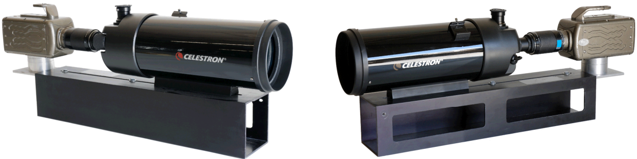
Figure 1. Opposing views of one of the camera and lens arrangement used in the laser trackers. The lens is a 2000mm refractive Celestron® lens attached to a 2X extender to achieve a nominal focal length of 4000mm. The camera is a Phantom V7 high-speed video camera.
