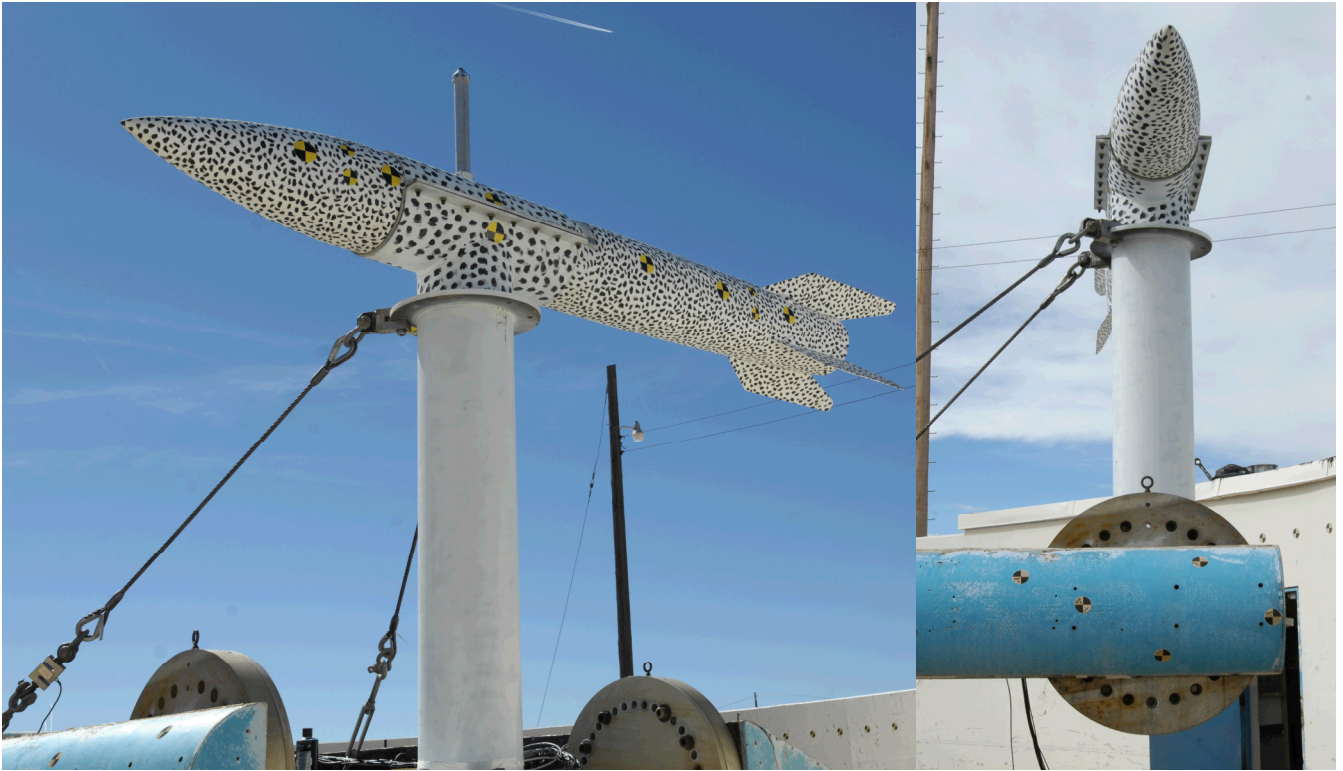
Figure 3. The left image shows the outboard quadrille markers on the test-unit. The right image shows some of the quadrille markers located on centrifuge arm. In the background of both images, some of the quadrille markers located centrifuge wall can be seen.
