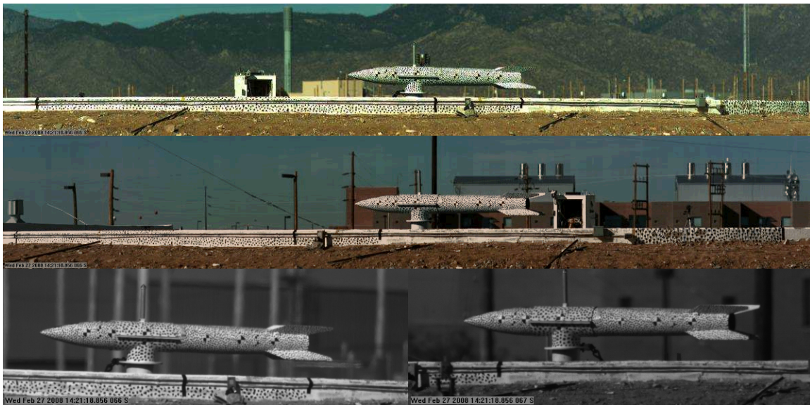
Figure 2. Sample images from stationary DIC left and right cameras (top and middle images, respectively) and images from left and right laser trackers (bottom two images).
