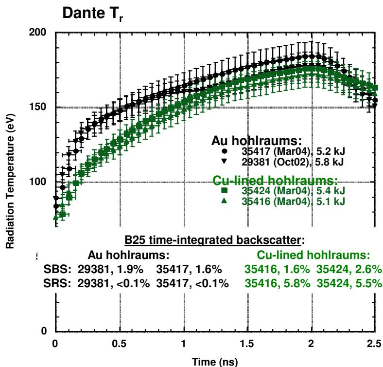
**\*Modification of a Laser Hohlraum Spectrum via a Mid-Z Wall Liner",**
