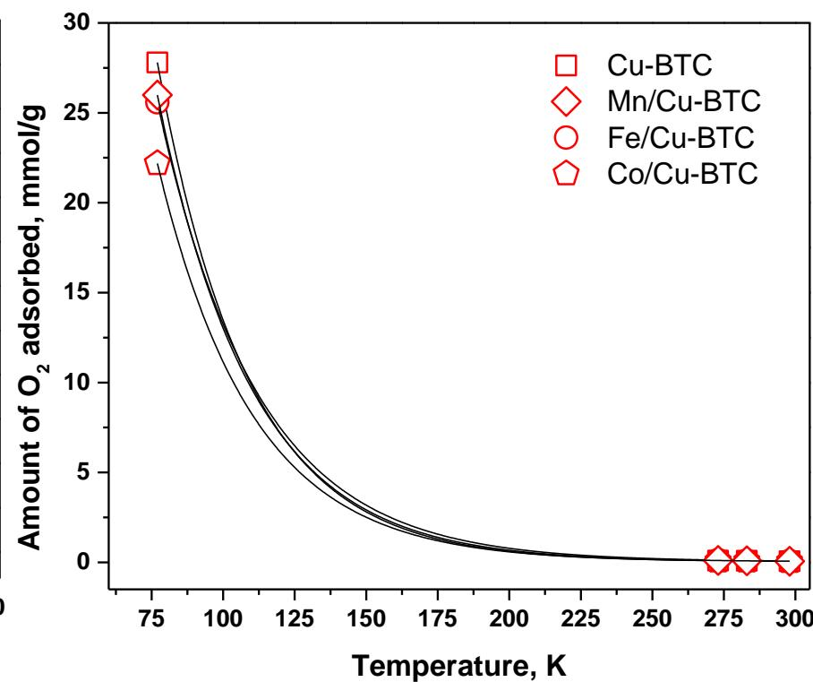
Distinct transition point temperature where the metal sites dependence on the  $\text{O}_2$  and  $\text{N}_2$  uptake is inverted
