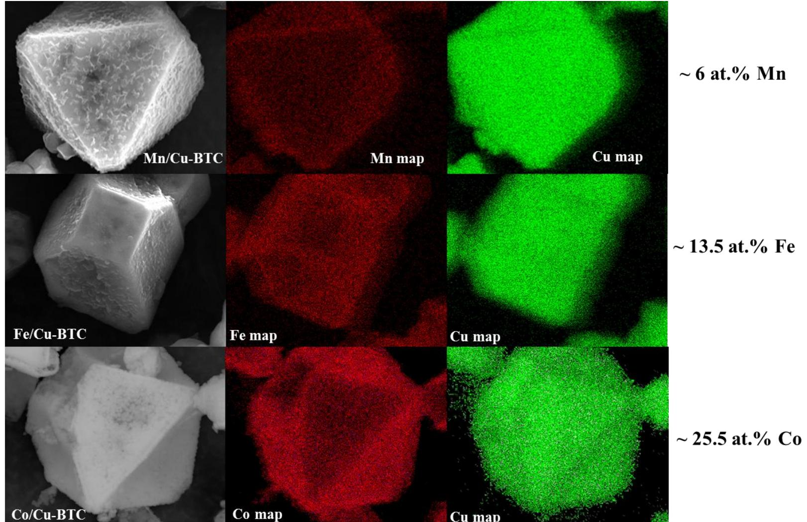
SEM-EDS mapping shows homogeneous dispersions of the substituted metals in the Cu-BTC matrix
