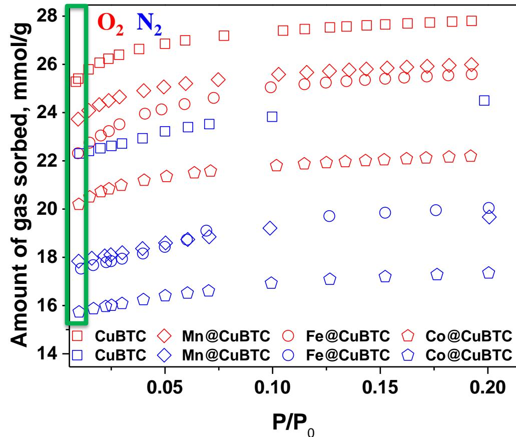
O<sub>2</sub> (red) and N<sub>2</sub> (blue) adsorption isotherms measured at 77K on pristine Cu-BTC and Mn-, Fe-, and Co-substituted samples
