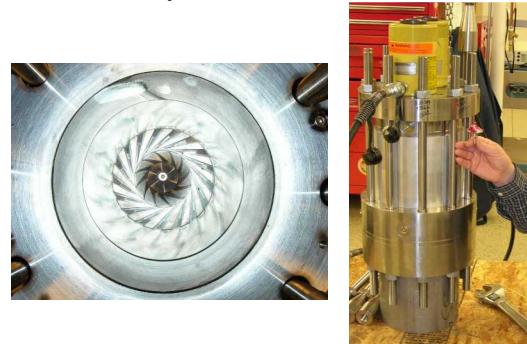
Figure 2: (Left) Main compressor (Right) SCO 2 turbomachinery.
