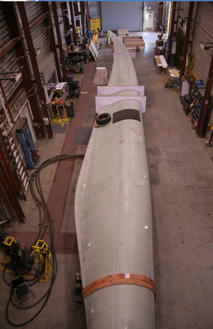
Structural Test of Knight and Carver Blade Test preparation of a swept blade providing twist-flap coupling for gust load reduction
